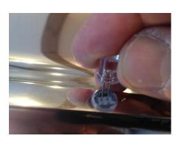
10. Turn reflector over and lift ballast tray to reveal diodes and adhesive.
