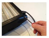
3. Remove 6 screws in end plate nearest the cord and remove end plate.
