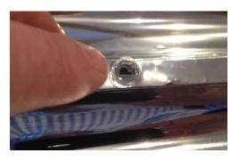
14. Insert white socket into clear holder from back of reflector.
