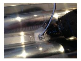
18. Slide reflector back into housing and re-assemble light.
