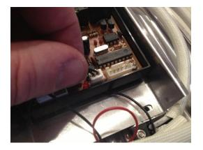
11. Use hot glue gun tip to soften and remove glue and old diodes.
