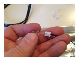
15. Install LED into socket.
