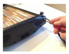
5. Pull reflector out part way with pliers.
